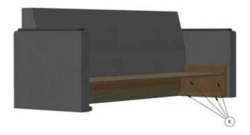
**K:** If the sleeper has optional End Frames, use a 7/16" wrench, or ratchet and socket, to unscrew the 4 bolts which secure the side frames.
